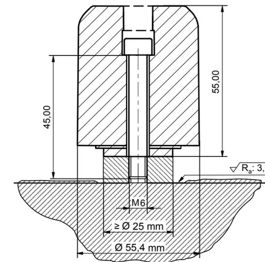
FAG SmartCheck installed with sensor mounting plate
