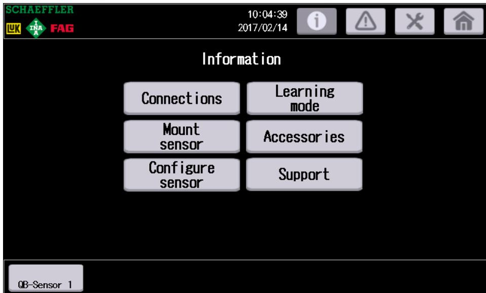
Here you can find information about the FAG SmartQB connectors, about assembly and configuration of the sensors and about learning mode. Lists of accessories and details of support are also available.
