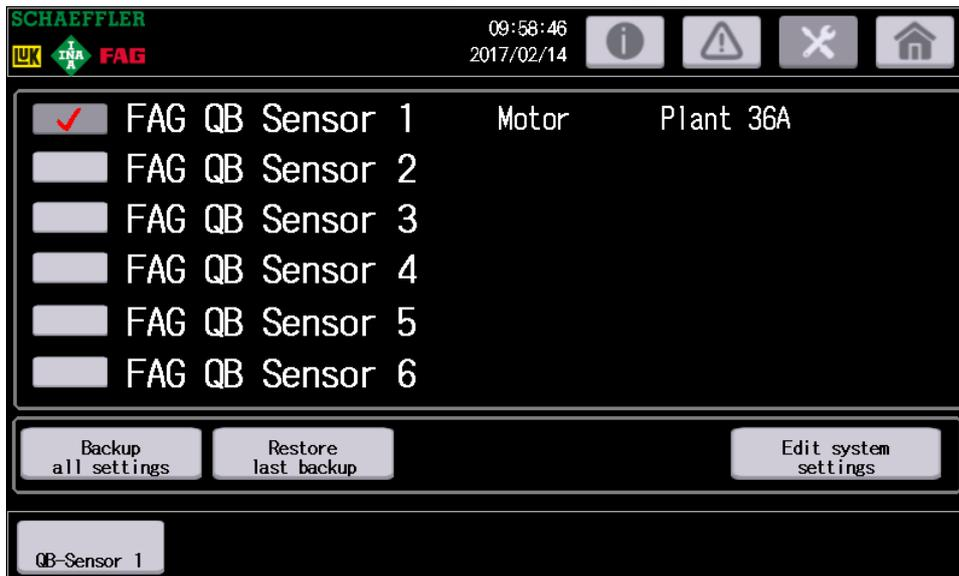
Tap on **Restore last backup** to read out the respective sensor settings.
