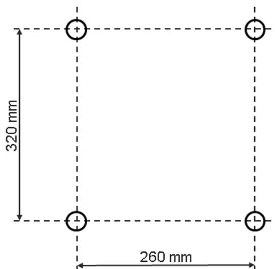
Use a drilling depth of 50 mm (or 10 mm longer than the length of the screws) for the fixing screws.
