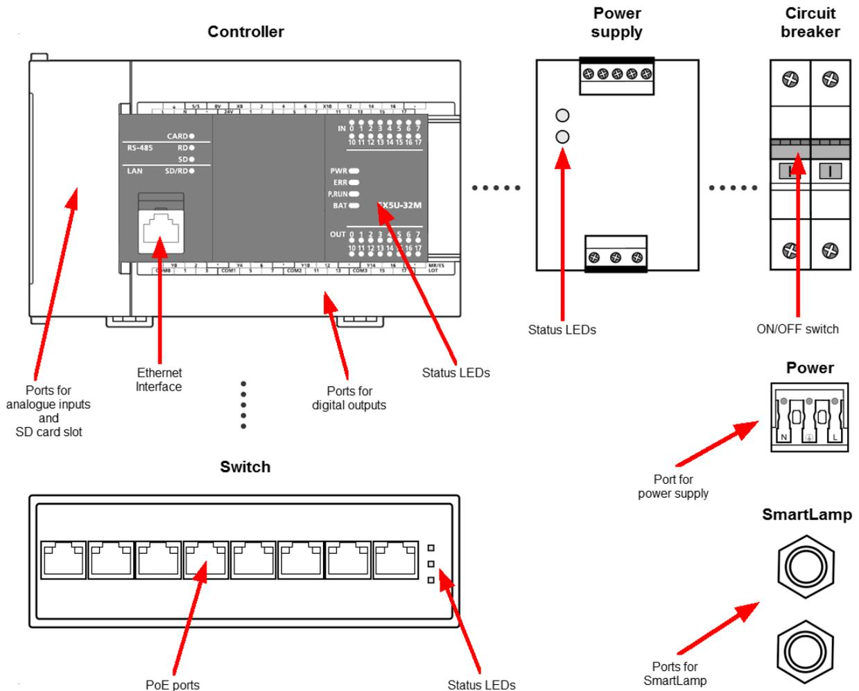
The FAG SmartQB features the following components and functions:
