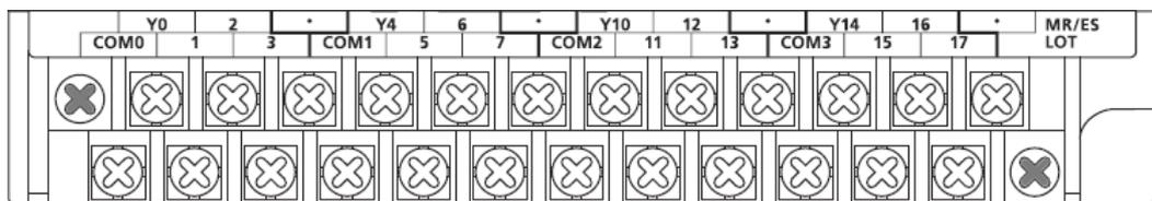
The digital outputs are arranged in groups of 4. Each group shares a port for the voltage to be switched. These terminals are indicated by "COM".
