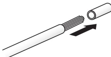
2. Push a ferrule onto the stripped end of the cable and firmly press it in place.
