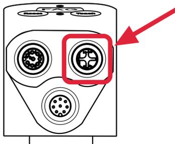
4. Lay the Ethernet cable to the FAG SmartQB housing.
