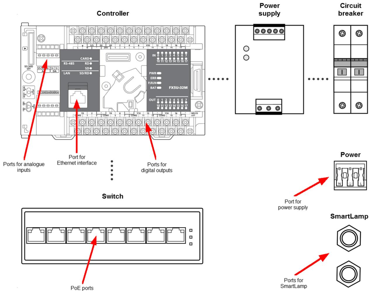
Details about the assignment of cables required for the analogue inputs [25](#), the digital outputs [26](#), the FAG SmartLamp and the power supply [28](#) can be found in the following sections.
